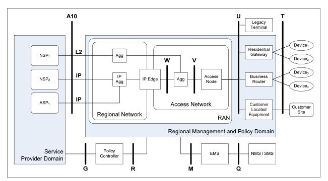
Figure 7 – Broadband Multi-Service Reference Model (from TR-144)
