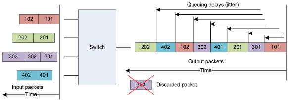
**Figure 5 – Congestion causing jitter and packet loss**
